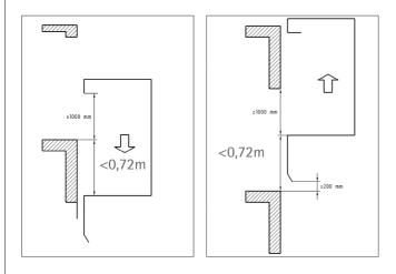
The structure of the system meets the requi-. rements of EN81-1:1998-A3:2009,chapter 9.11 and EN81-20:2014, chapter 5.6.7.
