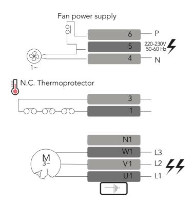
Motor Scheme A 2 Speed: AC2 with NC Thermprotector
