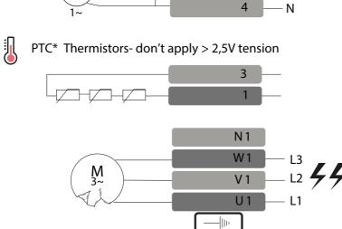
Motor Scheme B 2 Speed: MPV - with Thermistors PTC
