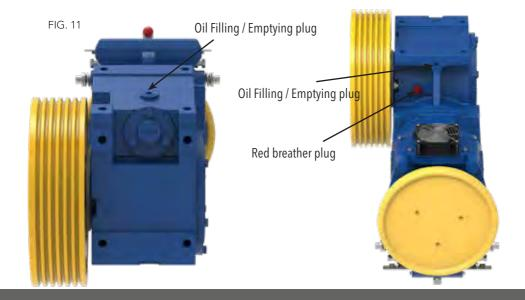
For each position of PENTA therefore, both horizontal and vertical, there is always a filler plug and a drainage plug.
