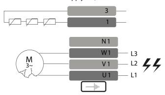
Connect the brake electromagnet using the relevant terminal board. (FIG. 12).
