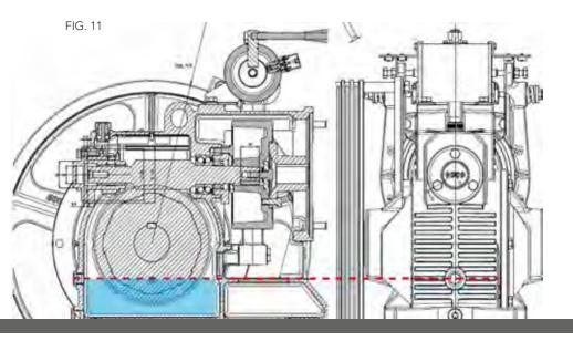
Check lubricant level periodically. Ensure there are no traces of oil on the brake pulley, brake shoes and traction pulley.
