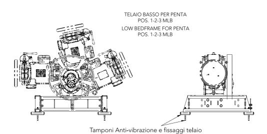
Anti-vibration buffers and bedframe fixing
