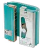
The BSG-25P is a bidirectional progressive safety gear used mainly for modernization applications. Certified in Wittur's UCM package but also as single component makes the BSG-25P also compatible with your UCM solution. The unique design allows up- & downwards gripping direction on the guide rail in contrast to other solutions which use the drive brake.
