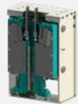
Single-direction progressive safety gear applicable for mid and high rise applications. Superb solution for car but also counterweight frame installation (modernization packages available). Brake pads from the automotive industry prevent wear on guide rails. Available for many global major elevator norms and directives.
