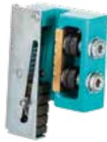
Braking force generated through a combination of disc springs and braking elements (adjustable by the disc spring assembly) activated. Simple and compact design for easy integration in different positions on car slings or counterweight frames. Low force needed to release after engagement.
