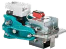
EBRA20 is an ascending-car overspeed protection (ACOP) and can be used also as UCM brake. The guide rail brake is installed on the car sling for modernization of existing elevators. Working as a standalone braking system, it only needs electrical tripping information (overspeed governor switch) to engage in case of overspeed. It does not substitute the safety gear for down direction.
