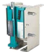
Single-direction progressive safety gear applicable for a wide range of loads. Superb solution for car but also counterweight frame installation due to reduced width dimensions (modernization packages available). Brake pads from the automotive industry prevent visible wear on guide rails. Available for many global major elevator norms and directives.
