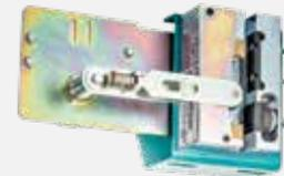
LADP is a bidirectional safety gear also available for heavy loads. Upwards braking power is applied through compression of a stack of adjustable disc springs. Downward progressive brake force is generated by deflection of adjustable leaf springs.
