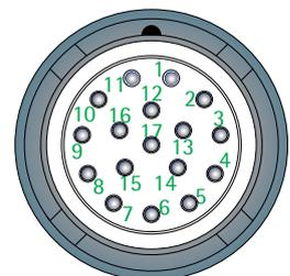
Pin contacts of signal coupling (exterior)
