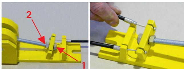
**Caution:** Mount Bowden cable symmetrically for round holders (see pictures below). Differences between 2 or 3 brakes must be considered!
