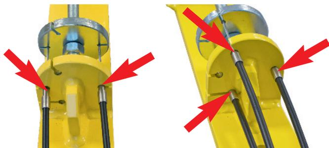
4. Insert the ends of the Bowden cables into the machine.
