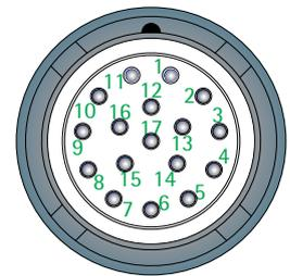
Pin contacts of signal coupling (exterior)
