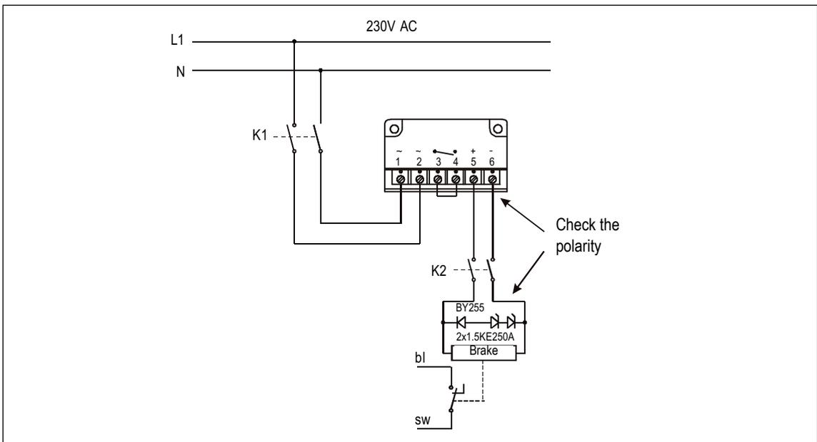
Fig. 5 Connection diagram for the BFK466 (circuit proposal for DC switching)
