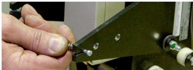
5. Then insert the sleeve ends. A certain amount of effort is needed, as the cables require some preloading. Note: The Bowden cables should be kept straight and not wound.
