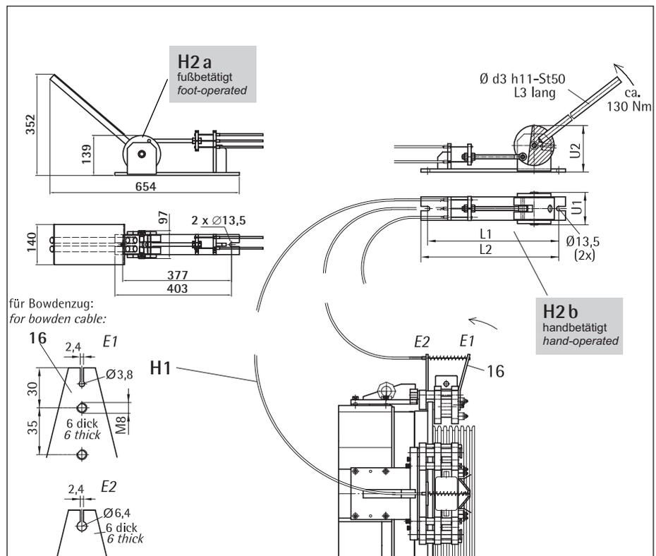
Release lever set with remotely controlled bowden cable
