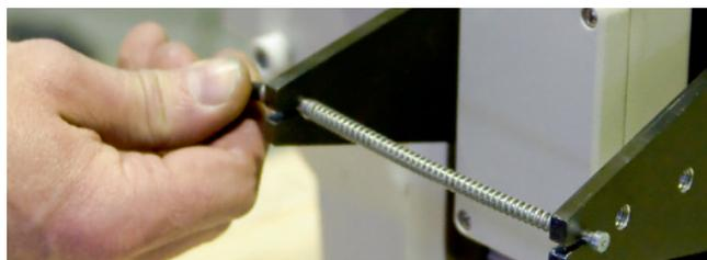
6. Preload the Bowden cables by turning the nuts on the stud bolts (2). The brakes must not yet release (check this!).
