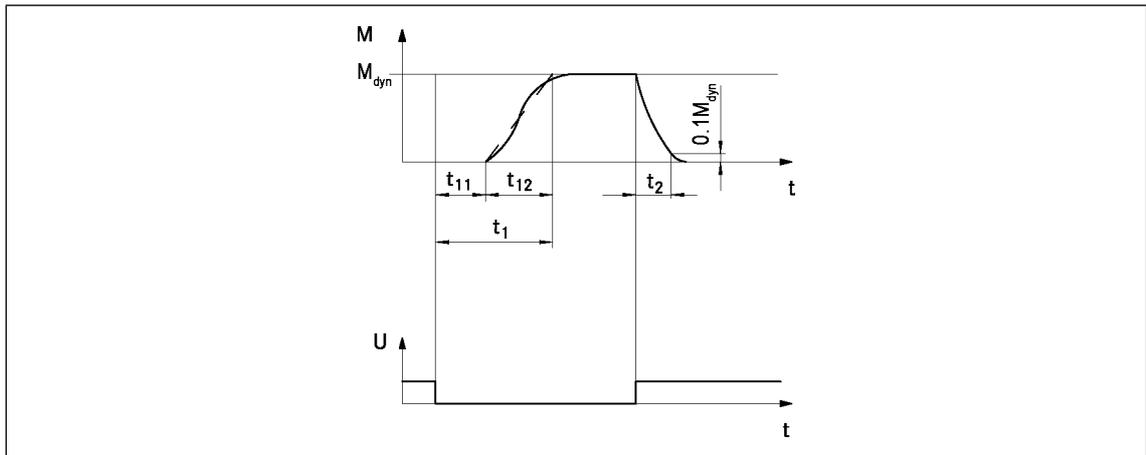
Fig. 2 Operating/switching times of the spring-applied brakes
