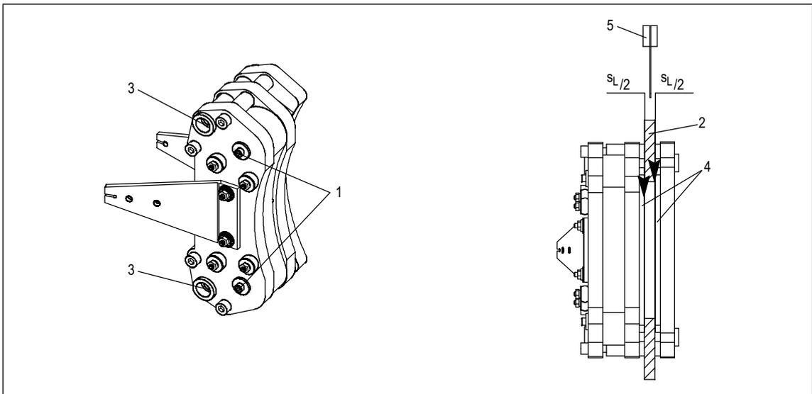
Fig. 4 Procedure for installing the BFK466-55 spring-applied brake
