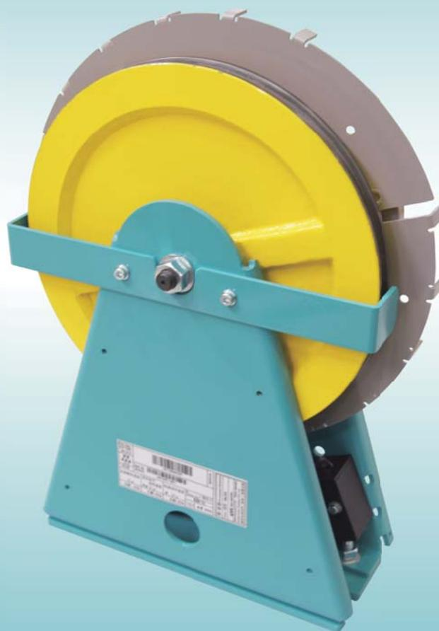
The OL25 detects overspeed by its flyweight mechanism and engages the safety gear on the entire circumference of brake mechanism.
