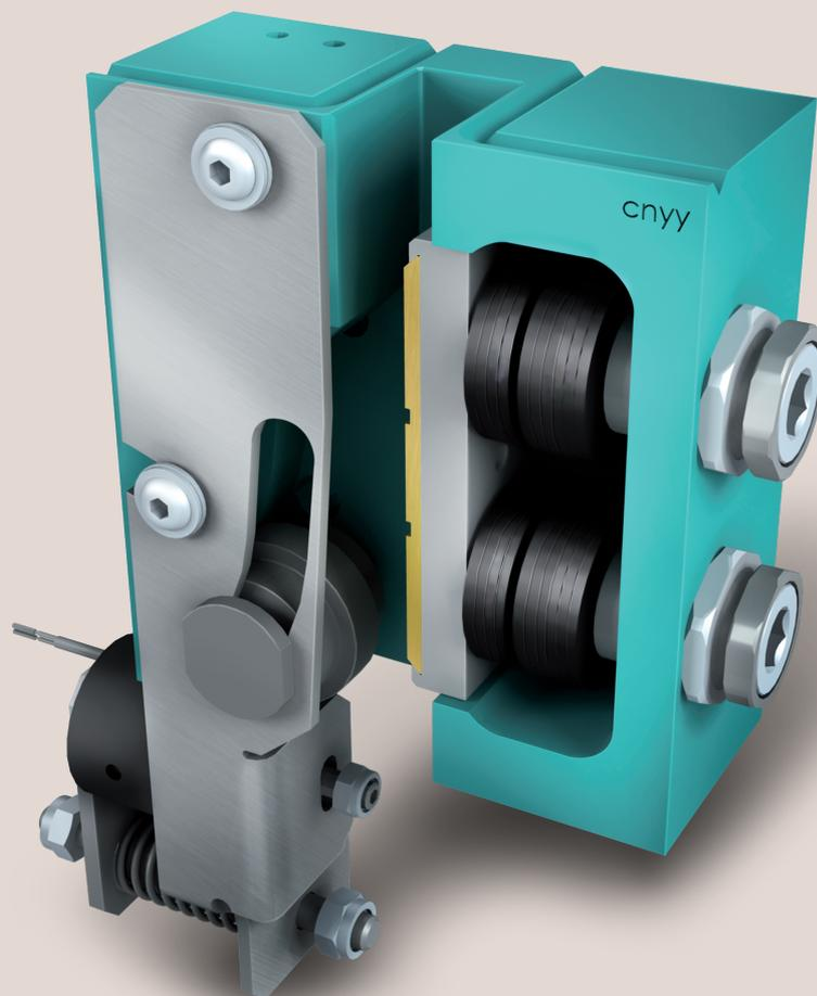
GLSG-22U is a progressive safety gear with mechanical and electrical components. Mechanical components are consisting of a combination of disk springs, braking elements and trigger mechanism with free movable roller.
