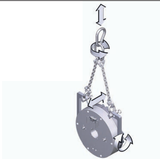
Fig. 8: Lifting mechanism for hooking onto a hoist
