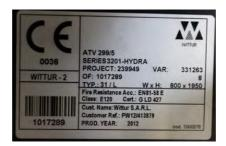
Likewise, you can also find on the label essential information such as: the door type, the clear opening, the high opening and motorization type.
