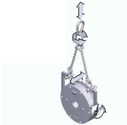
Fig. 8: Lifting mechanism for hooking onto a hoist
