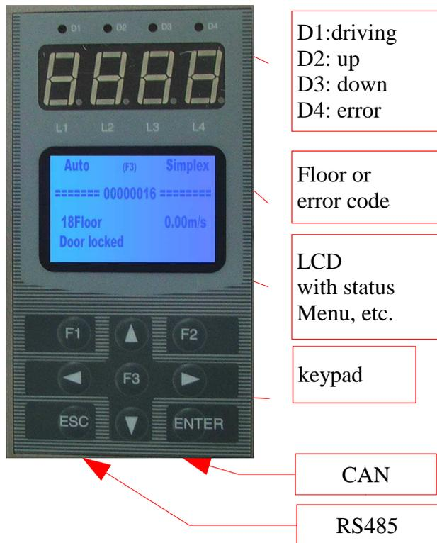
Optional a control element can be directly inserted on board F5021B, or the external control element can be connected with a special cable with the 9pin Sub-D-linkage JP15. The USB-plug of the cable have to be plugged in the left plug (RS485). A plug-in into the right plug by mistake arose no claims, the control element is just not working.
